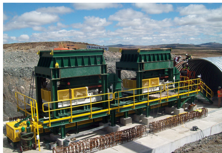
Apron Feeders are prepped for installation. These will carry ore from the stockpile through underground tunnels
