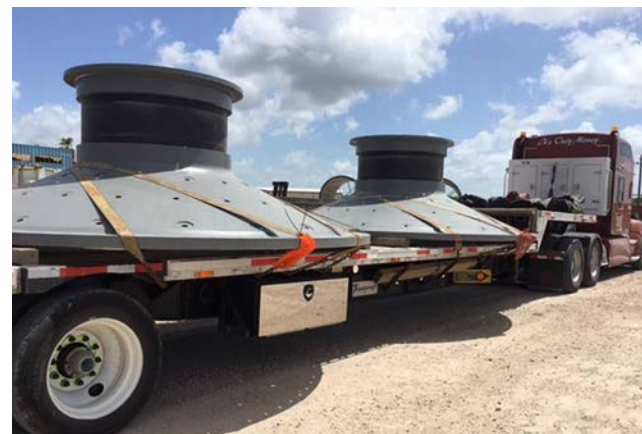
CFI saw the arrival of a major piece of equipment this month. A ball mill – which is used to grind and blend materials – was shipped to facilities over two deliveries. Seen here is the head feed for the mill.
