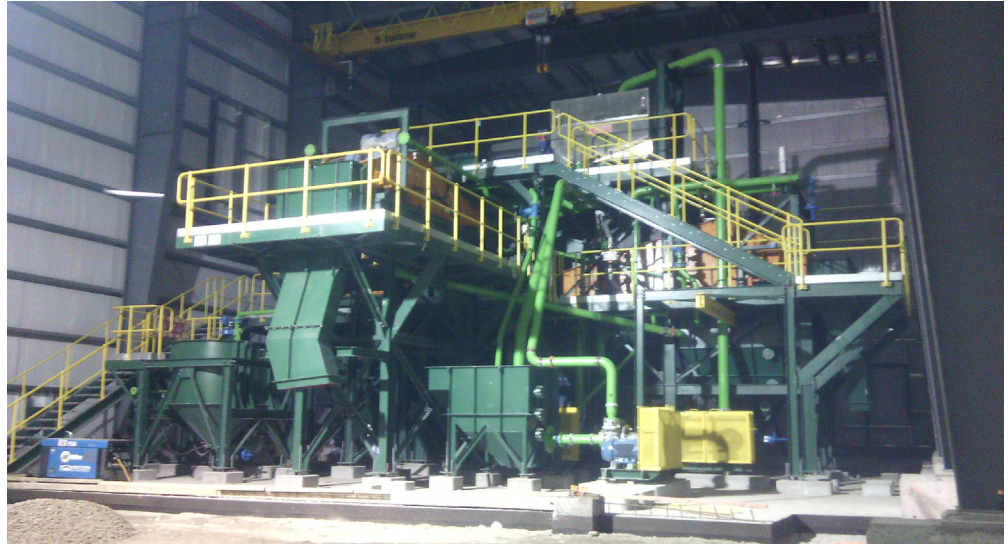
CFI's Dense Media Separator (DMS). Work on the DMS was completed in January. The DMS will help separate fluorspar from other minerals.
